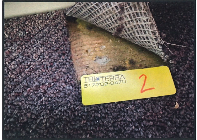
Photo #:2 Material #: 2 Non-ACM Subject: View of Carpet Adhesive. Located under carpeting throughout.
