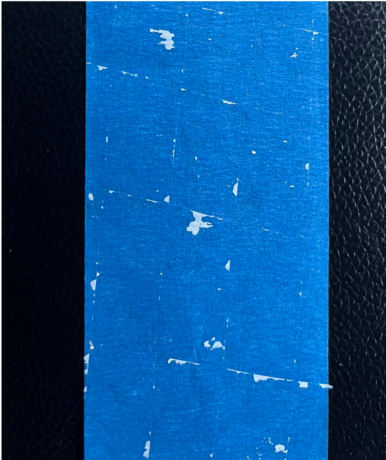
Figure 5: Results from cross-cut adhesion test with SW extreme bond primer.
