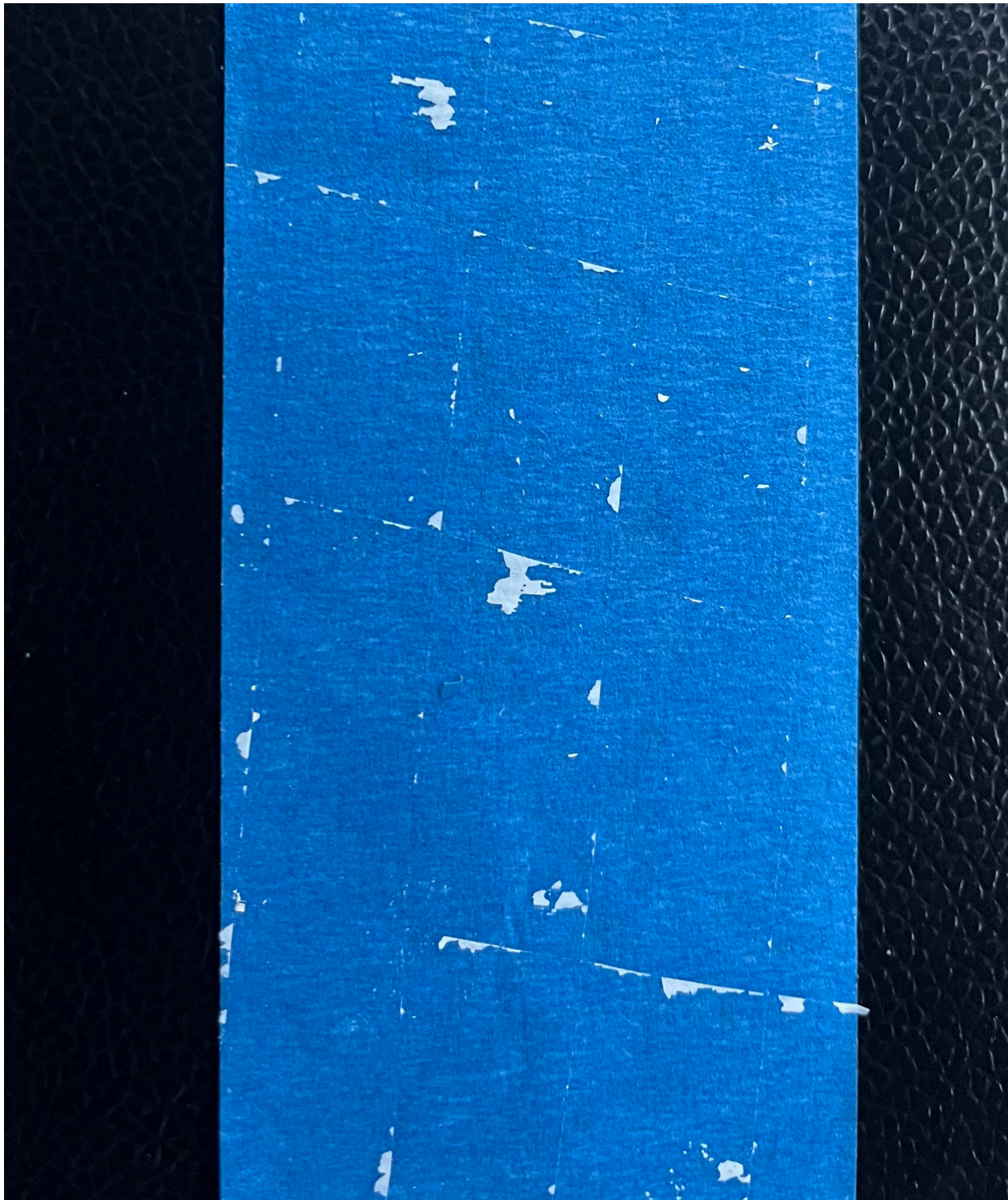
Figure 5: Results from cross-cut adhesion test with SW extreme bond primer.
